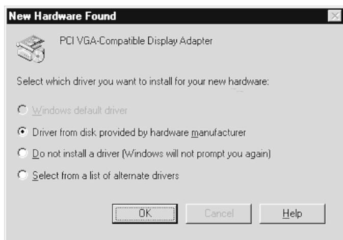
Integral recommends installing the drivers provided on the *FlashPoint 128 Display Drivers Disk*. If you wish to proceed, Select “Driver from disk provided by manufacturer” and click OK.
